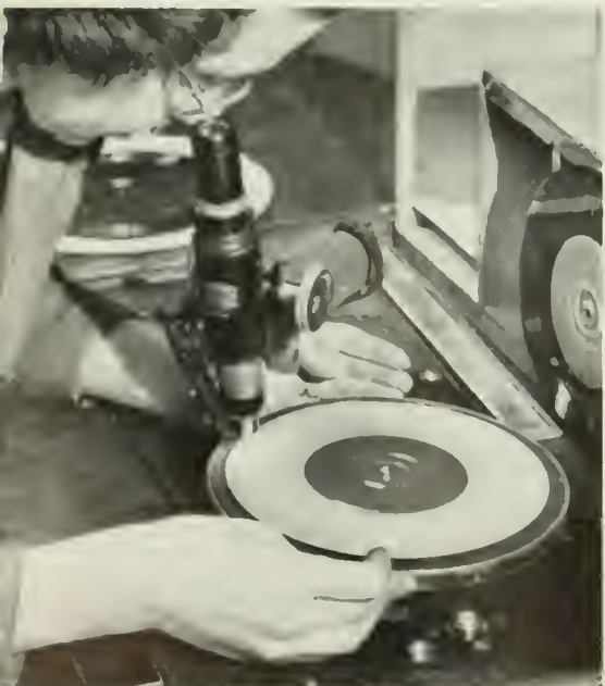
5 Exact centering of a 45-rpm record is assured by checking the movement of the outer rim under a microscope.
